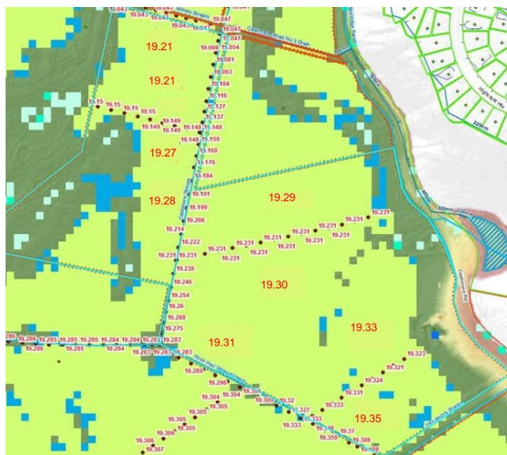
Figure 2. Spot height 200-year flood levels (Shown as the larger red numbers) provided by Council, Heathcote Model at 564 Cashmere Road, Christchurch
