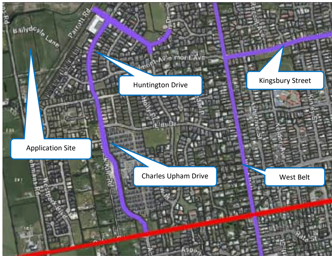
Figure 3: Rangiora Road Hierarchy Map (Purple roads represent Urban Collector Roads, red represents strategic roads and rest are local roads)
