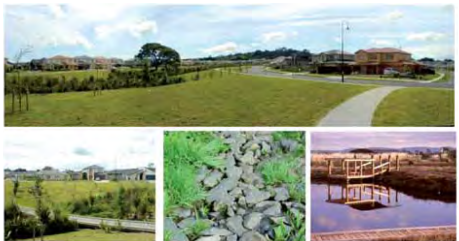
Examples of blue network responses that focus on also improving local settings. These often result in increased levels of amenity and property value, greater surveillance and hence greater safety levels. Approaches that focus on slowing the movement of water also help reduce the risks of flash flooding and erosion/coastal degradation.
